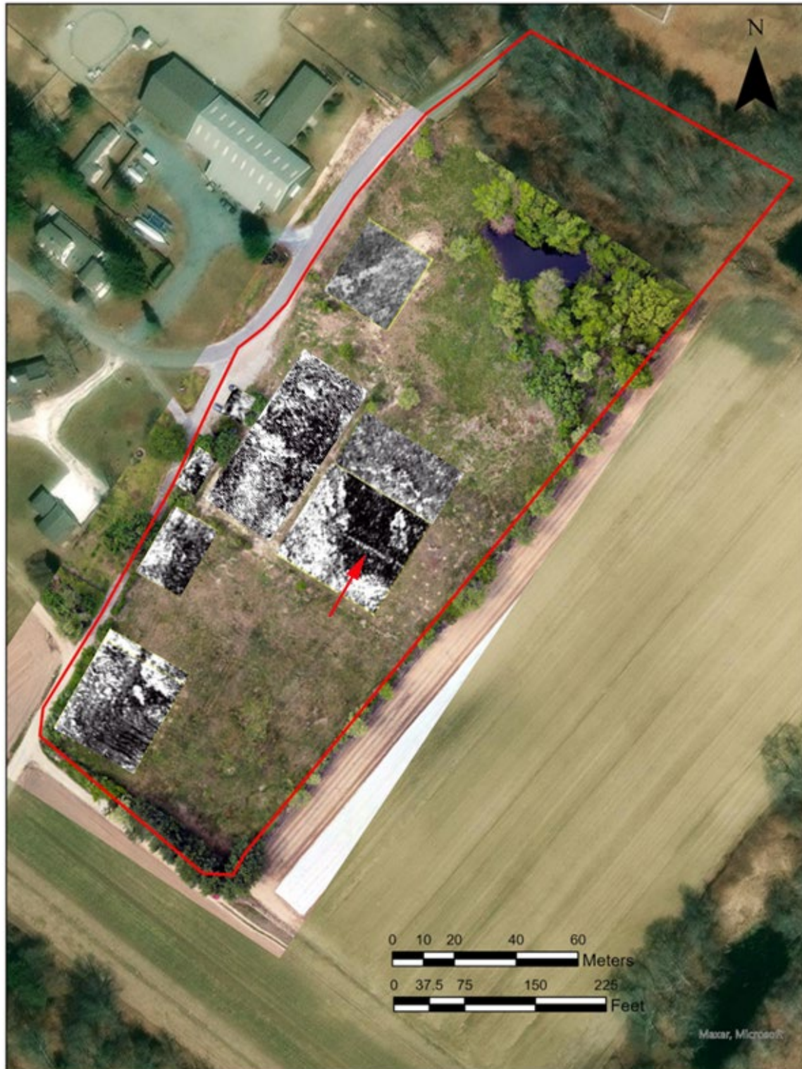
Map 6: Aerial photograph of Lot 3A showing the GPR amplitude maps showing the data at approximately 24 centimeters below surface. Note the linear anomaly on the summit (red arrow).
